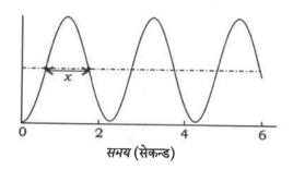
The unit step response of a unity feedback system exhibits sustained oscillations as shown in the figure below. The open-loop transfer function of the system is  $G(s) = \frac{K}{(s+1)(s+4)(s+a)}$ . The time x in the figure is 1.0471 second.
